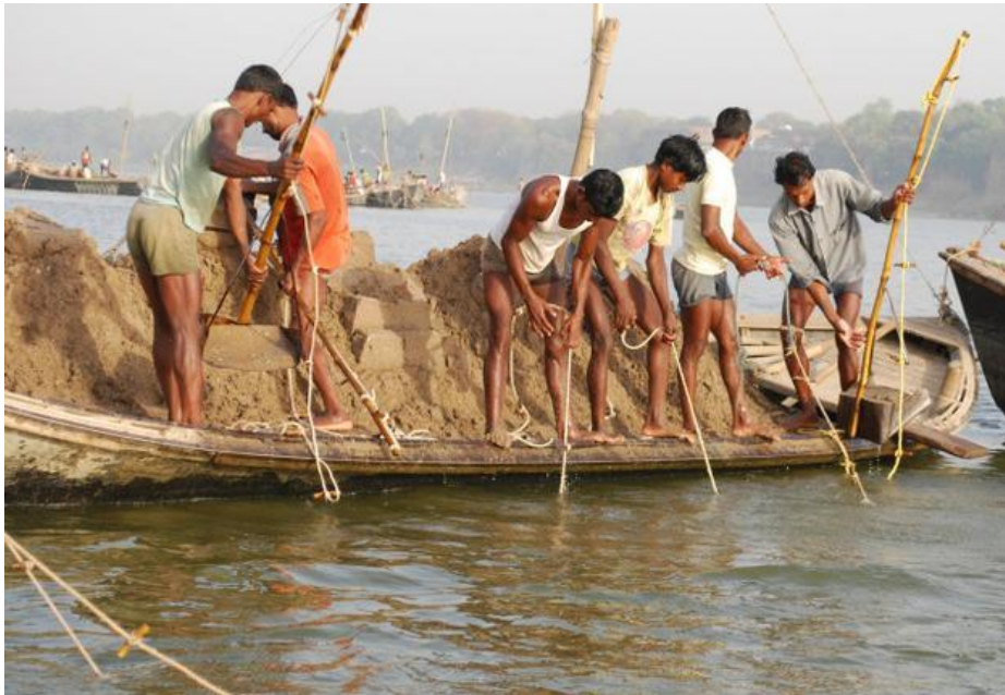
Figure 2.4: India: manual wet river sand mining from boat
